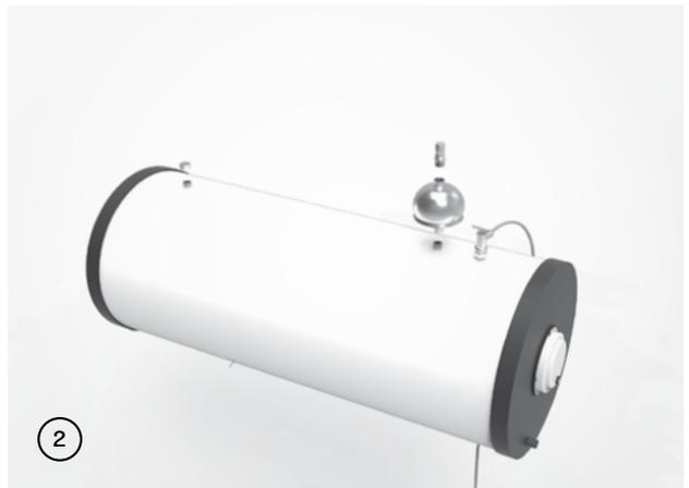
2. When the closed circuit is completely filled, seal both the safety valve and the plug. It is highly recommended, in order to achieve the device's optimal operation and efficiency to install an expansion tank on the closed circuit too. The expansion tank will absorb excess pressure and restrain the liquids of the circuit. As a result, they will not be rejected from the heater because of vaporization.
